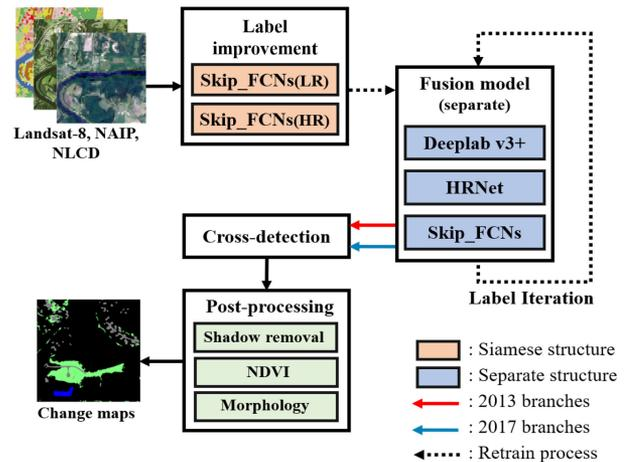
Fig. 3. Flowchart of the overall scheme.
