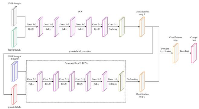
Fig. 8. Overall framework for generating classification and change maps.
