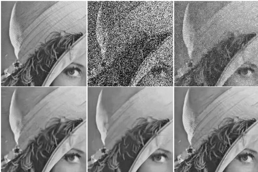
**Fig. 3.** Lena images recovered by the five PR algorithms at SNR = 20 dB. For comparing clearly, the parts of the images are presented. From left to right and top to bottom: the original image, the image recovered by WF (PSNR = 10.93 dB, FSIM = 0.8967), DOLPHIn (PSNR = 21.36 dB, FSIM = 0.9819), BM3D-prGAMP (PSNR = 31.94 dB, FSIM = 0.9972), SPAR (PSNR = 31.82 dB, FSIM = 0.9966), and ConPR (PSNR = 33.51 dB, FSIM = 0.9985).
