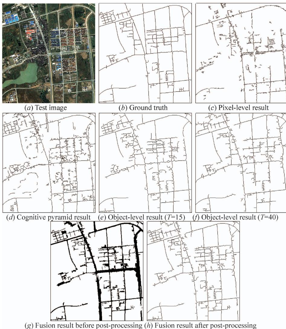
Figure 3. (a) A suburban test image (400 by 430 pixels with 4-m spatial resolution). (b) The ground truth road network. (c) and (d) Road maps for pixel-level and multiscale cognitive pyramid approaches, respectively. (e) and (f) Object-level results for a single scale ( $T=15$  and 40, respectively). (g) and (h) The multiscale fusion results before and after post-processing,
