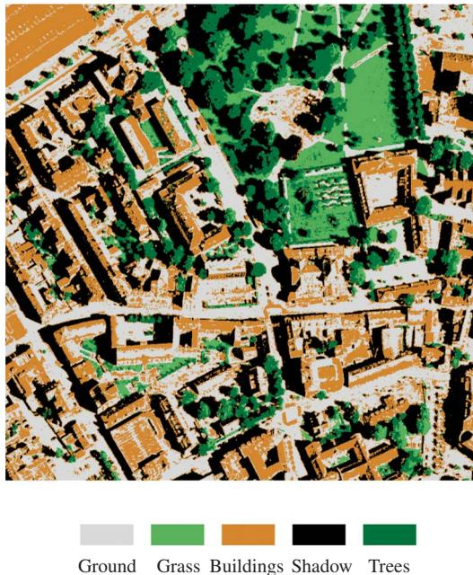
Figure 3. Map of spectral-only classification obtained by performing SVMs on the aerial image (overall accuracy = 82.5%).
