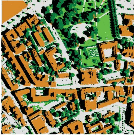
Figure 6. Classification map for soft re-classification approach with Max-Min feature (overall accuracy = 95.0%).
